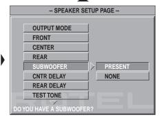
The SPEAKER SETUP PAGE provides setup items relating to surround sound and bass management of the audio signals at the analog outputs of the RDV-1060.
